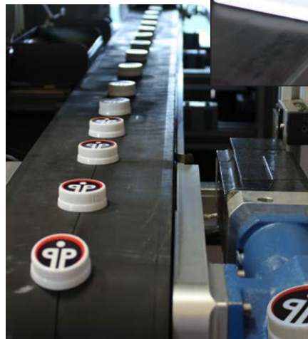
▲ This inkjet system is capable of printing 45,000 bottle caps per hour with CMYK, in a single pass. Conveyor feeds parts directly into a counter/accumulator packaging system
